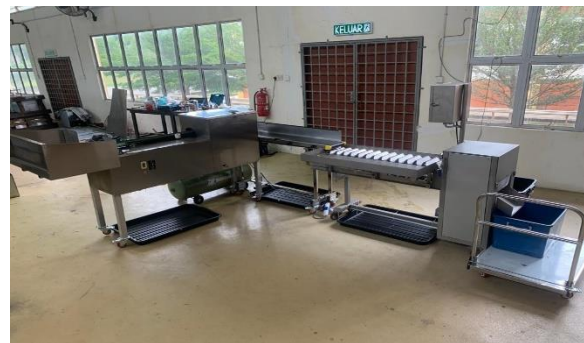
An invented semi-automatic fish gut removal and fish the head-cutting machine
