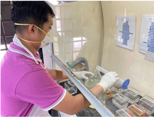
Figure 1. Preparing dilute nitric acid under fume hood for mercury decontamination purpose (credit: Hizat and Idham)
