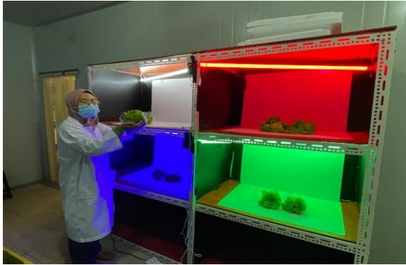
The setup of LED treatments, installed in the 5°C walk-in chiller
